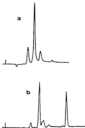
Fig. 3. Chromatograms of blue dyes extracted from pieces of material. The detector was set at 600 nm. (a) Cloth dyed with Dispersol navy B-T; (b) cloth dyed with a mixture of Dispersol navy C-4R and Dispersol green C-6B.
